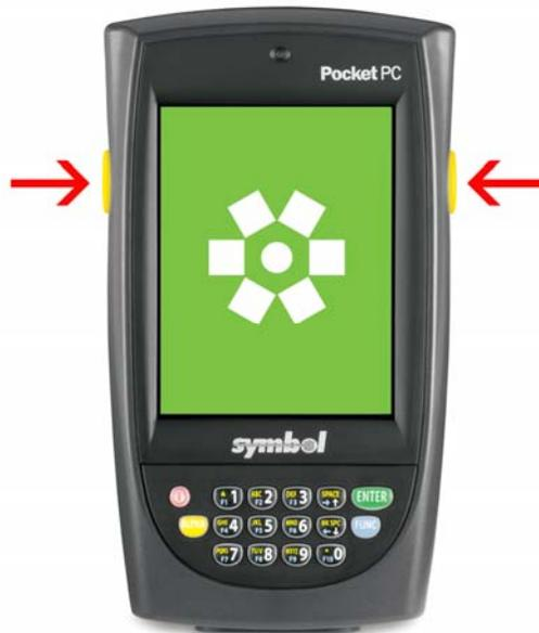
Hold the unit 2 to 4 inches from the barcode when scanning. Holding the unit too close to the barcode may not register properly and holding the device too far from the barcode could cause inadvertent scans (especially if scanning from a sign-in sheet or list).
